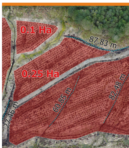
Aerial photos used with GIS to accurately measure planting preparation operations
